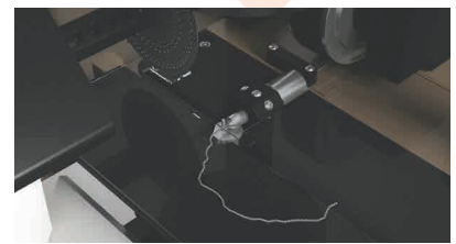
⑥ Bending Wire Bending Machine Starts Bending
